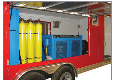
Fully Enclosed Breathing Air Trailer with Fill Compressor, Air Storage Cylinders and Containment Fill Station
